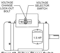
Figure 17. Voltage Change Switch (115 VAC Position)
